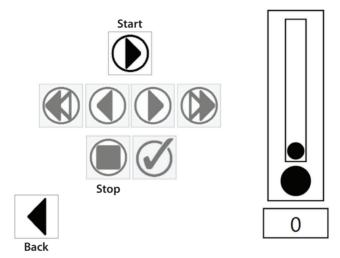
Attach a flow meter to the pump and then click on the **start** button to start the calibration.
