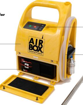
Easy to use control panel with highly visible OLED display
